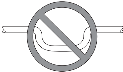
Fig. 22 - Insufficient Condensate Trap
